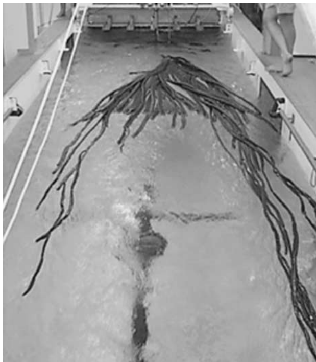
Figure 2. Experimental setup of the drag tests on Durvillaea in a flume (Human Performance Centre, Dunedin, NZ). The specimen of D. antarctica shown had an approximate length of 7 m and was reduced in ‘bulkiness’ as part of the lamina had been lost due to wave action and only a few but very long strips of the lamina remained.
